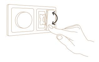
Place the rocker loosely on top of a switch. Make sure the rocker is aligned into the center of a switch. Now gently push the rocker from the center until you feel a "click".
