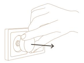
Grab the knob from two sides and then pull the knob off the saft. It may require to use force to get the knob off the shaft. Important is to pull the knob evenly from two sides. NB! Do not use screwdrivers or other similar tools to remove the knob!
