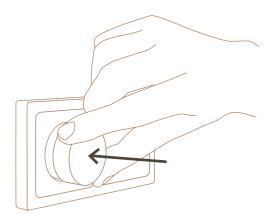
Place the knob loosely on top of a shaft.
