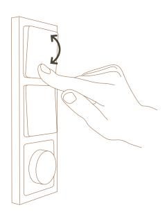
Place the rocker loosely on top of a switch. Make sure the rocker is aligned into the center of a switch. Now gently push the rocker from the center until you feel a "click".
